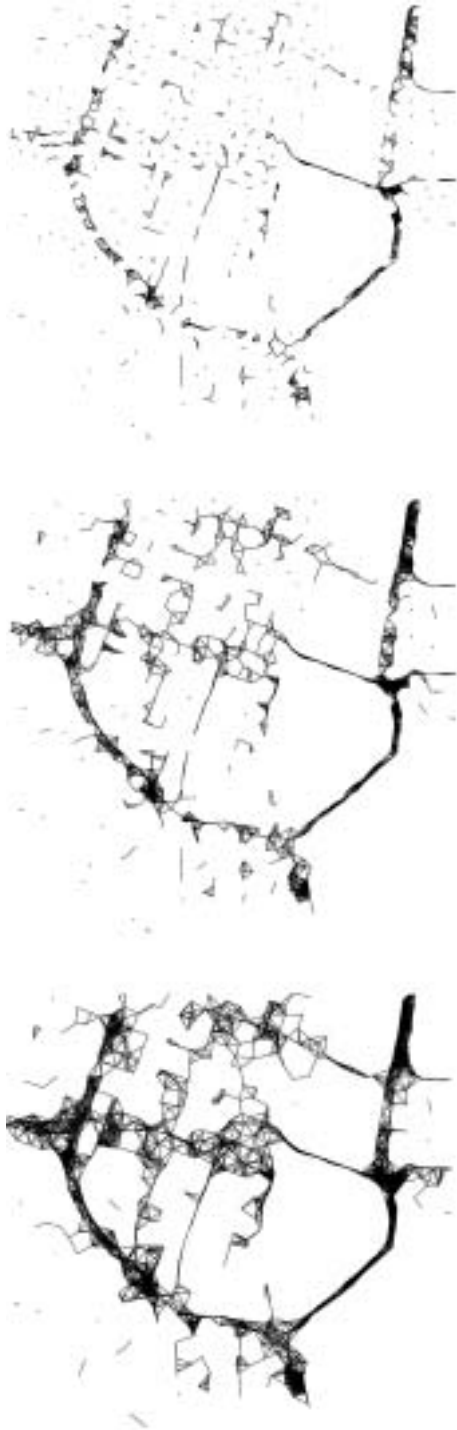
Fig. 6. Three graphs resulting from different connection radii on the same set of node positions. From top to bottom, the radii are 50 m, 75 m and 100 m. Notice that even with an unreasonably large range, there are still many components in the interior of the network.
