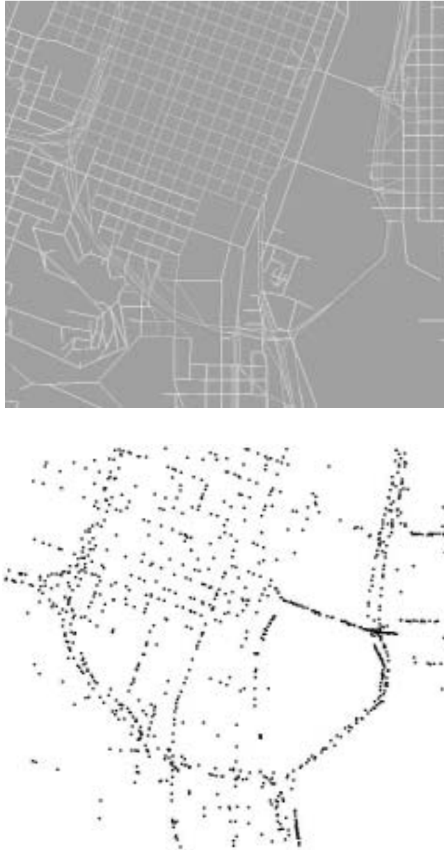
Fig. 4. The upper panel shows the road network on which vehicles are moving, and the lower panel is a snapshot of those vehicles at 7 am in a TRANSIMS simulation of Portland, Oregon. The gap on the right of each figure is the Willamette river.
